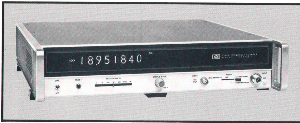
Fig. 1. Model 5340A Microwave Frequency Counter can measure 10 Hz to 18 GHz automatically, using only a single input. Eight digits are displayed. Resolution is selectable from 1 Hz to 1 MHz.
